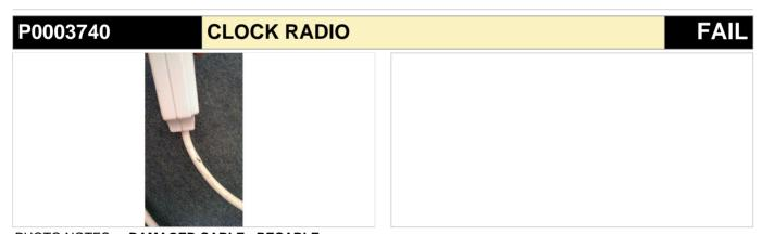
PHOTO NOTES: DAMAGED CABLE - RECABLE
